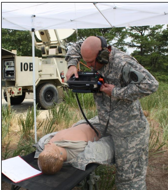
A medic utilizes a man-portable physiological monitoring device with streaming video, voice and photo capability to send medical information to doctors for real-time communication and decision making. (Photo by Edric Thompson)
